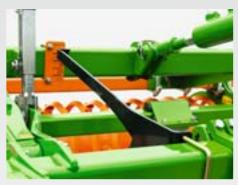
The depth setting is carried out mechanically as standard via the turnbuckle or there is the very comfortable, hydraulic adjustment from the tractor seat enabling a response to different soil conditions on the move.
