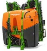
UF 1602 mounted sprayer with 28 m Super-S2 boom
