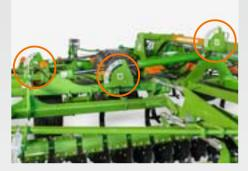
Both the front compact disc harrow along with the tine section and the levelling unit can be equipped with hydraulic depth adjustment. Any adjustments made are easily visible from the tractor seat via the three large scales.
