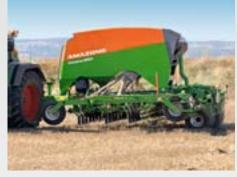
Thanks to the lower link attachment, integrated running gear and hydraulically folding wings, the Cayena is an impressively compact and manoeuvrable unit.
