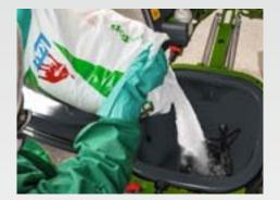
For inducting powders or granular spray agents, an additional mixing nozzle is positioned underneath the suction aperture which safely prevents any blockage of the suction aperture. This mixing nozzle can be steplessly adjusted for intensity.
