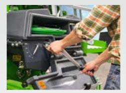
Independently of each other, both the coulter pressure on the TwinTeC coulters and the seed placement depth are adjusted in the SmartCenter. Thanks to the use of the universal tool these centralised settings are done quickly and easily.
