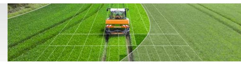
Automatic part-width section control of up to 128 part-width sections
