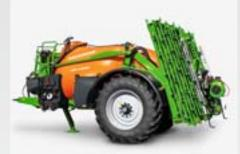
Alternatively, the Super-S2 boom, from 15 m to 28 m, can also be used on the UX. All booms can be automatically controlled with DistanceControl parallel to the target surface.
