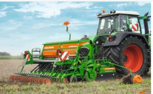
The universal all-round combination for behind-the-plough and mulch sowing: KG rotary cultivator, KW wedge ring roller, AD with RoTeC Control coulters.
