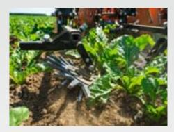
In addition to control between the rows, mechanical weed control within the rows is also important. In this respect, the aggressiveness of the tool, e.g. a finger hoe, must be able to be tailored to the growth phase of the row crops.
