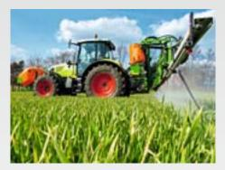
The special advantages of easily-manoeuvrable tractors in smaller fields and the better control in sloping conditions are strong arguments for the front tank solution.
