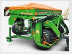
The blower fan for seed delivery is driven by a hydraulic motor.
