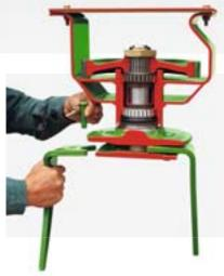
Quick change tine system for rotary harrows and rotary cultivators: The tines are simply pushed into the sockets of the tine carrier and secured with a lynchpin. There is no easier and faster way.
