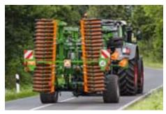
The integrated running gear provides the machine with a high manoeuvrability both, on the road and in the field. Depending on country-specific traffic regulations, an allowable 40 km/h fast road transport speed is possible.
