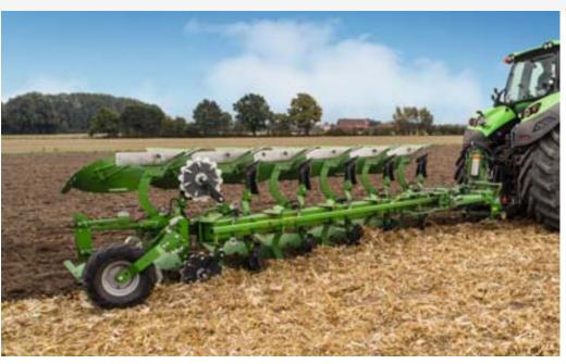
One specific quality feature of the Cayros ploughs is the heat treatment with the ©plus hardening process for the mould-boards. This heat treatment results in a prolonged longevity, high impact strength and a smaller pulling power requirement and thus reduced fuel consumption.
