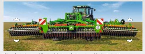
This perfect soil contour following ability is yet further enhanced by the ContourFrame system. Here, the hydraulic rams of the outer sections are pre-pressurised via hydraulic accumulators and then, when moved into the float position, it means that each of the three sections can adapt upwards and downwards to follow the soil contours – even in hilly terrain.
