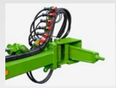
The Cenius-2TX is coupled to the tractor via the lower links, a towing eye or a K80 ball coupling. This flexibility allows its use on tractors with caterpillar tracks or centre pivot steering as well its use on standard tractors.
