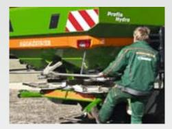
The robust rolling and parking device for the ZA-V and ZA-TS eases both the coupling and the uncoupling of the spreader and when manoeuvring it around off the tractor when in the yard. The castor wheels are quickly folded in and out and optimally protected against dirt.
