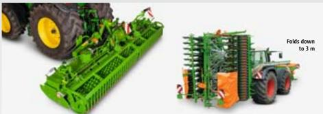
The rotary cultivator in 4 m, 5 m and 6 m working widths folds hydraulically down to a 3 m transport width and is suitable for tractors up to 265 kW (360 hp). The main gearbox on the folding rotary cultivator is equipped with a 2-speed lever change for rapid adjustment of the tine speed to different soils and working intensities. The well-laid out, compact design of these extremely robust folding rotary cultivators makes them perfectly capable of high outputs, even in smaller fields.
