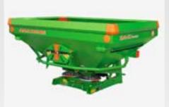
The optimised steep walls of the twin hopper allow an even flow of fertiliser – even on slopes.
