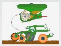
Decisive is the modular separation of grain singling and grain planting. The precise pneumatic singling of the seeds is performed via the centralised singling drums for six or eight rows.
