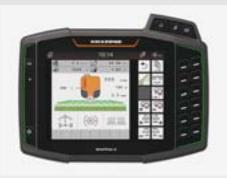
The AmaTron 4 operator terminal supports, for example, the precise switching in 50 partwidth sections, automatic boom lowering at the start of application, automatic documentation and the part-area, site specific application rate control.
