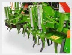
Optionally, for both rotary harrows and rotary cultivators the soil can be loosened in the tractor wheel marks with the height and side adjustable eradicator tines. The wheel mark eradicators are equipped with a sprung overload safety device to protect against damage.
