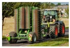
Safe road transport with a transport width of less than 3 m is assured by the main frame which is hydraulically folding as standard.
