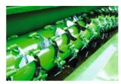
For the Groundkeeper and Profihopper ranges there is the SmartCut exact cut rotor that offers outstanding collection qualities. The outstanding feature of the SmartCut rotor is the special v-formation blade arrangement which leads to both a reduced fuel consumption and noise level.
