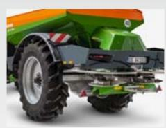
Over-sized tyres reduce the ground compaction and make operation possible even under the most difficult of conditions. Tyres with a cleated AS profile can be specified with a track width from 1.8 up to 2.25 m.
