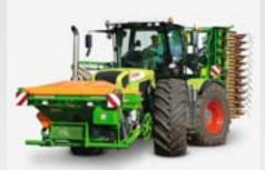
The front mounted seed hopper has been designed to be wide and low so as not to obstruct the driver's view. The same applies to the rear visibility for an uncluttered view of the rear mounted implements.
