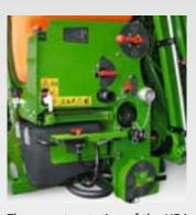
The operator station of the UF is located on the left hand side of the machine. Only three operating taps are sufficient for the actuation of all functions.
