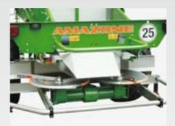
The ZG-B models have a universal spreader unit for the application of earth-moist materials (lime) up to 15 m and mineral fertilisers up to 36 m spreading width.
