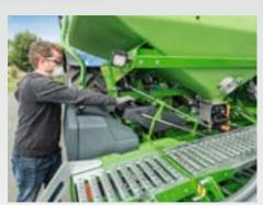
For calibration the driver pushes the calibration tray via a rail from the side to underneath the metering housing and opens the calibration flap. Either via the calibration button or TwinTerminal the calibration procedure can then be started.
