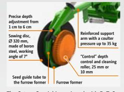
The Cataya Special is equipped with RoTeC Control coulters with a spacing, from choice, of either 12.5 cm or 15 cm. The basic sowing depth can be set directly at the coulter in 3 different positions.
