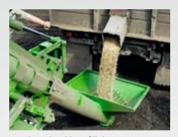
In order to be able to fill the Primera DMC with both seed and fertiliser, AMAZONE offers a hydraulically-driven filling auger. Using this system the filling time is kept down to just 15 minutes meaning that the output of the drill is even further extended.
