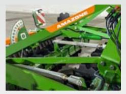
The working depth adjustment of the disc segment can, from choice, be carried out mechanically or, for more comfort, hydraulically on the move from the tractor cab.
