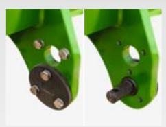
When attached to the tractor, the machine is coupled to the lower links via Cat. 3 pins. However, by simply reversing the pin in the lower link journal, a spacing of either Cat. 3 or Cat. 2 can be achieved.
