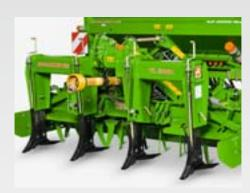
The compact TL deep loosener loosens and inverts the soil. This enables AMAZONE to offer one-pass cultivation without ploughing, even where high levels of straw prevail.
