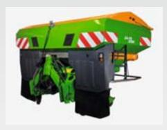
The additional mud flaps on the ZA-V and ZA-TS ensure that no dirt is thrown from the tractor wheels onto the spreading discs.
