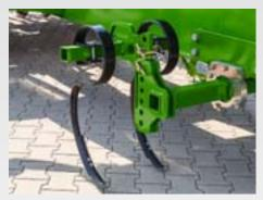
For operation on loose or poorly reconsolidated soils, wheel mark eradicators are available as option. The wheel marks are loosened and levelled. By hydraulic actuation, the lowering and lifting is carried out automatically on the headland or when folding for transport.
