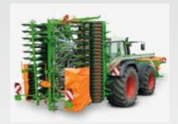
The Avant is available as rigid version in 4 m and in a foldable version up to 6 m which folds down to a transport width of 3 m for road transport.
