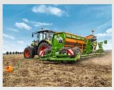
The D9 6000-TC "Combi" trailed seed drill with a 6 m working width is perfect for precise behind-the-plough and mulch sowing. High surface area coverage is guaranteed with a tank capacity of 2800 l for fertiliser and seed and working speeds of 15 km/h.
