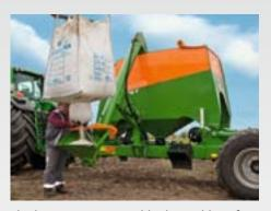
The large openings enable the problem-free filling of the hopper via a front end loader. However, on request, the machines can also be equipped with a filling auger.
