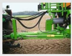
A tracking, universal, straight or hitch drawbar with hydraulic steering prevents wheel track damage. A braking system is available on request.
