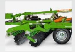
The front discs distribute the organic matter by intensively cutting and mixing the crop residues on the soil surface. At the same time, a finely crumbled structure occurs within that top soil layer.
