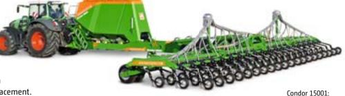
wide in the field, narrow on the road with 3 m transport width
