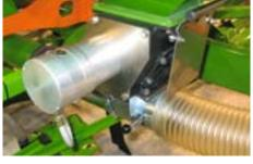
With the full electric metering drive, a precise regulation of the seed rate is made possible.
