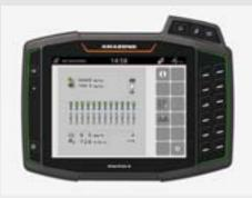
The professional level of electronic equipment offered, coupled with an ISOBUS terminal, ensures the comprehensive monitoring of the machine and its convenient operation.
