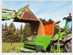
An especially-wide loading board, accessible via folding rear steps, simplifies the filling of the seed drill. The very spacious fill opening dimensions allows the quick and convenient filling process - not only from big bags and front end loader buckets but also from sacks.
