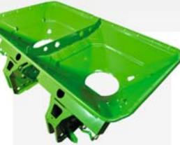
The base hopper of the ZA-V and ZA-TS is deep pressed and is without corners, edges and weld seams. This provides a continual and even distribution of the fertiliser.
