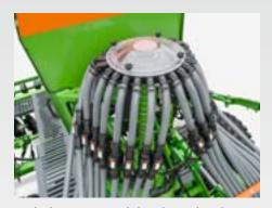
With the segmented distributor head, asymmetrical tramlines on one half of the machine can be carried out without any undesired seed rate reduction on the other machine half. With the segmented distributor head, electric half-side shut-off and Section Control are possible.
