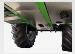
With its covered-in chassis, the UX Super provides, even in high crops, an ideal solution to optimally protect both machine and plant. Thanks to the underbelly cover, the complete implement underside is encased in stainless steel plates so that chassis and plants are optimally protected.
