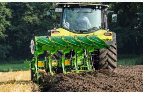
The headstock is equipped with a one-piece lower link cross shaft which has very good shock absorbing properties and in this way significantly reduces the load on the tractor's rear lift linkage. This is enabled by two pivot bearings, one on each side of the lower link cross shaft, which effectively absorb the shock loads generated.
