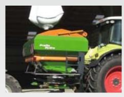
The hydraulic-operated roll-over cover with the ZA-V and ZA-TS enables you to continue spreading even when the weather conditions turn against you.
