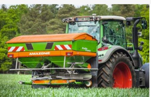
ZA-V 2000 Profis Tronic weigh cell spreader with Limiter V<sup>+</sup>
