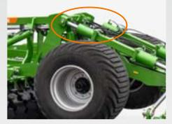
The angle of inclination of the Certos can be adjusted by means of a hydraulic upper tie bar. If the machinery pulls to one side, it can be easily compensated for from the driver's seat in the tractor cab.
