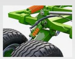
The optionally available step-less hydraulic depth control enables the adjustment of the working depth whilst on-the-move to react to varying soil conditions and operational conditions.
