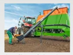
The TAM filling auger for the Citan large area seed drill and for the Condor tine seeder can be controlled without any problem via a spool valve on the machine. The transport dimensions remain under a height of 4 m and a width of 3 m.
