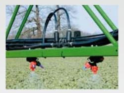
The pressure re-circulation system (DUS) for all AMAZONE sprayers ensures that the concentration of spray chemical at the nozzle is always constant. When cleaning, the system is flushed with clear fresh water right up to the nozzle.
