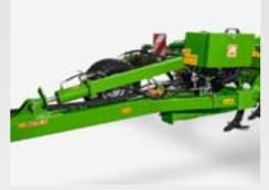
As an option, a selectable traction system is available. When activated, it additionally transfers part of the machine weight back on to the rear axle of the tractor with up to 1500 kg being available at a maximum working depth.
