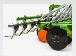
Independent of soil conditions and weather, the RoTeC pro Control coulter enables sowing at higher speeds. The sowing depth is set quickly and comfortably via the coulter pressure. The settings on the coulter allows the precise readjustment for deep sowing operation.
