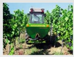
In the vineyard, the spreader's narrow overall width of just one metre prevents damage to the vines.
