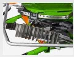
For spreading adjacent to fields, roads or water courses, the ZA-V can also be equipped with the electrically actuated Limiter V<sup>+</sup> which is available as an option. Then the border spreading device can be smoothly lowered into the fertiliser flow to the desired height.
