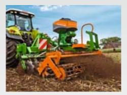
As part of the metering system, underneath the seed hopper, is the seed shaft where all seed types and seed rates can be sown using either the normal or fine seed wheels provided. The drive to the seed shaft and fan are carried out with an electric motor and hydraulically respectively.
