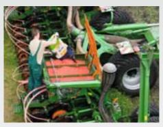
With a working width of 9 m yet only 2 seed hoppers have to be filled. This centralisation means shorter filling and set-up times and thus results in an additional increase in efficiency.
