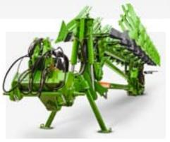
Particularly convenient is the parking position of the Hektor in its transport position. As the tilt adjustment does not have any influence on the position of the lower link cross shaft, the coupling and uncoupling of the plough on and off the tractor is particularly comfortable. The lower link cross shaft is, from choice, available in either Cat. 3 or Cat. 4N.
