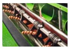
On all EDX machines, the adjustment of the stripper fingers is carried out simultaneously for all the rows. As a special option, electric remote control of the stripper finger is available, enabling the driver to regulate the stripper finger position via the AmaTron 3 in the tractor cab during operation.
