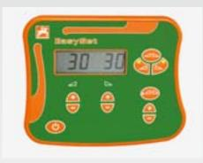
With the aid of the EasySet operator terminal, the spread rate shutter apertures can be electrically set via key pressure independently of each other to either side and can be readjusted on the move. This also allows the rate to be individually adapted to the left and right hand side.
