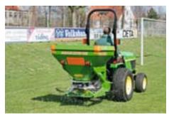
With minimal expense, the E+S winter application spreader can also be equipped for spreading granular fertiliser. It produces an excellent lateral and longitudinal spread pattern as well as achieving high work rates.
