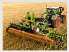
The Catros-2TS in working widths of 4 m to 6 m is equipped with a bogey chassis and drawbar. In the field, its performance is characterised by a very smooth run because the running gear is swivelled completely above the frame.
