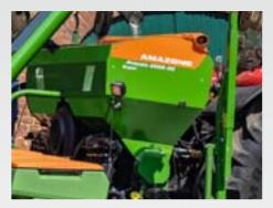
The fertiliser hopper can be installed with a capacity of 950 l or 1250 l depending on the model and level of equipment. The Precea-CC precision air seeder can be combined with Double-Shoot under-root fertilisation.
