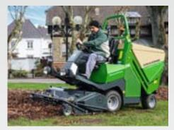
Thanks to the superb suction effect almost "everything" (leaves, chestnuts, acorns, etc. ...) is collected and the hopper capacity is optimised. In addition, the chopping up of the leaves by the rotating blades speeds up their decomposition.
