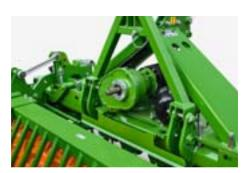
Via the PTO shaft through-drive, a mounted implement, for instance such as a pneumatic seed drill, can be driven.
