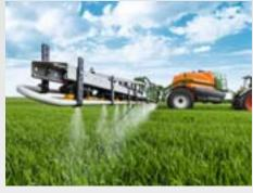
Due to the specific profile design, AMAZONE booms are at the same time superbly light and superbly strong. The working widths of the booms of 21 to 40 m allows the optimum matching to farm sizes and structure.
