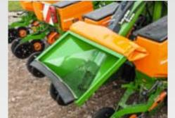
For filling the ED with fertiliser, AMAZONE offers a hydraulically-driven filling auger, integrated within the machine concept. In this way fill times can be reduced and the work rate of the machine further increased.
