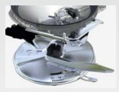
Due to its large aperture, the ultra-modern spreading system on the ZA-V can achieve application rates of up to 390 kg/min. The hopper tip, which tapers down to the shutter slide, prevents any residues being left making the machine easy to clean.
