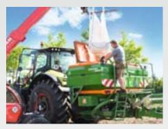
The XTender features a pressurised tank with a capacity of either 2200 l or 4200 l, which can be split in a ratio of 50/50. Application rates from 2 to 400 kg/ha can be achieved. Thanks to the large hopper opening, filling is quick and simple to accomplish.
