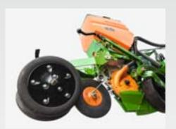
The AMAZONE Contour sowing unit is ideally suited to both mulch sowing and when working after the plough. The outstanding feature is the optimum soil contour following via the depth guidance rollers and the longitudinal tandem.
