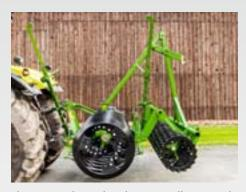
The optional NRP breaker ring roller is available as a following roller to give a more intensive levelling and crumbling effect.
