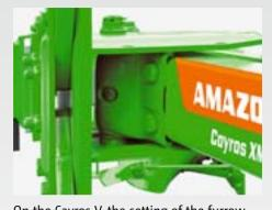
On the Cayros V, the setting of the furrow width is carried out steplessly and hydraulically from the tractor cab. Needless to say that the system is so sophisticated in design, that the traction point and the furrow width are also correctly adjusted at the same time.
