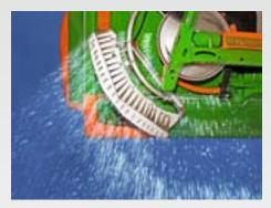
When side, boundary or water-course spreading using the hydraulically-actuated Limiter border spreading device, it is not necessary to either stop the spreading operation or to leave the tractor.
