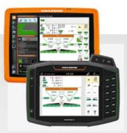
With the practical and cleanly arranged AmaTron 4 or AmaPad 2 ISOBUS operator terminal only one terminal is required to control all the different fertilising functions. All the relevant data is clearly displayed.
