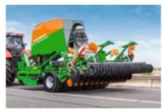
With the Matrix tyres, which have been especially developed for the Cirrus, the machine, even when completely filled with seed, can be safely transported on the road at up to 40 km/h where national road traffic regulations allow. Coupling to the lower link arms ensures the superb manoeuvrability of the Cirrus, for instance on the headland.
