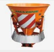
The EK-S mounted spreader is ideally suited for the reliable operation in winter salt application. With its working widths of up to 8 m and hopper sizes of 150 to 370 l, it is perfect for medium application rates.
