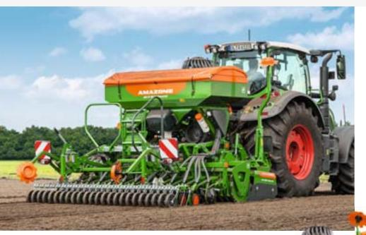
The metering unit of the AD-P Special is driven electrically allowing calibration by the press of a button and the very simple adjustment of the seed rate from the tractor cab. The easy accessibility simplifies the exchange of the metering cassettes and calibration.
