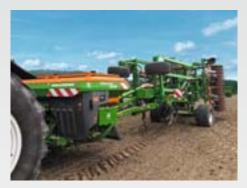
Via the 3-point linkage (Cat. 3/4N), the XTender is mounted onto the tractor with a favourable centre of gravity. The coupling of the following implement onto the Xtender is also carried out via a standardised Cat. 3 or 4N lower linkage
