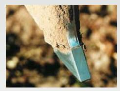
The hard-faced, "on-grip" chisel openers create a clean seed furrow into which the seed and fertiliser is placed – tried and tested 100,000 times over!
