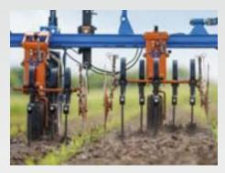
Hoe rollers protect sensitive crops from being buried by soil and guarantee optimum growth. Nevertheless, plants benefit from the additional nutrient mineralisation provided during hoeing.
