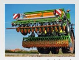
For transport or at the headlands the seed drill is pulled forward with the aid of the "Liftpack" system to reduce the lifting power requirement.
