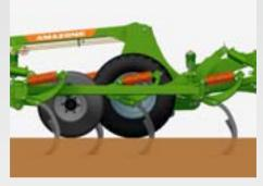
To ensure that the machine runs smoothly, also at the larger working widths, and operates at a constant depth, additional pressurised support wheels are integrated into the machine from a working width of 6 m. Again, to loosen the tracks of these wheels, a tine is also fitted behind each wheel.
