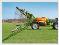
The parallelogram suspension of the UX enables spraying heights of 0.5 m to 2.5 m to be achieved. The boom position is excellent in all directions due to optimum co-ordination of the suspension system.
