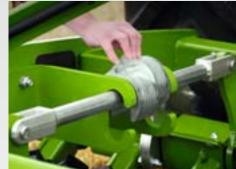
The working depth on the Catros Special can be comfortably adjusted by swivelling in and out spacer plates that are arranged centrally to the left hand side of the machine.
