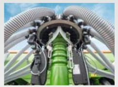
The segmented distributor head is arranged behind the seed hopper directly above the coulters. Half-side shut off of the Centaya Super via the segmented distributor head is also possible, for instance in asymmetrical tramlines at the field's edge.
