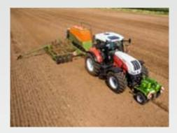
The front T-Pack U intermediate axle packer rolls the area in the centre of the cultivation disc segment. In this way, the soil in front of the machine is again additionally reconsolidated which is of benefit on light soils. The pre-running T-Pack U intermediate axle packer can also be operated as a front packer in solo operation.
