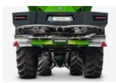
The sheet metal is manufactured from highquality steel to withstand the abrasion caused by the fertiliser. The ZG-TS high-performance trailed spreader comes with a mechanical spreading disc drive, whereas the ZG-TS Hydro has hydraulically-driven discs.
