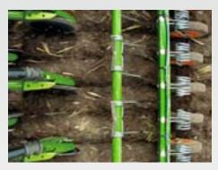
The large distance between the rear and front row of coulters ensures blockage-free sowing. With only one cutting disc per coulter, AMAZONE ensures blockage-free material passage, even with a 12.5 cm row spacing and mulch sowing at high speed.
