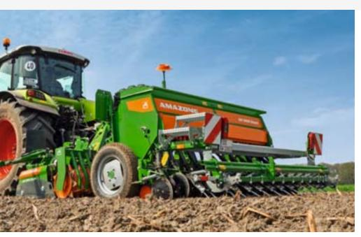
D9 3000 Super with Exact following harrow in combination with rotary harrow and tooth packer roller
