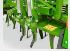
For operation on compaction-sensitive soils and at a reduced working depth, the optionally available tractor wheel mark eradicators make sense. They loosen the packed wheel tracks behind the tractor tyres.
