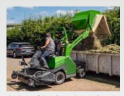
The design of the collection hopper allows the emptying at a height of 2.1 m (Profihopper 1250 SmartLine) or 2.5 m (Profihopper 1500 SmartLine). The point of delivery has been positioned far to the rear so that even high-sided containers can be filled as well as possible.
