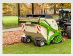
Because of the strong suction effect produced by the rotor, the Groundkeeper can also be used for collecting mowed grass, leaves, twigs, acorns, chestnuts etc.
