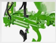
The hydraulic NonStop stone safety release features, in principle, one hydraulic cylinder per plough body with each one directly connected to a nitrogen-filled hydraulic accumulator. After having negotiated the obstacle, the plough body is automatically returned into position.
