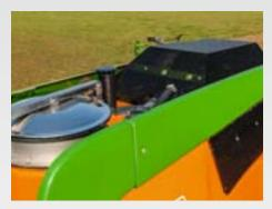
As from the new model year, the Pantera will meet emission standard 4. With regard to the topic of post exhaust emissions treatment, AMAZONE relies on the exhaust gas recirculation with a diesel oxidation catalyst and diesel particulate filter – all of which help in saving the environment.
