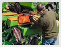
The seed hoppers hold 55 l. The pressurised tanks can be opened with one hand and are protected by a rubber lip against dust ingress. Furthermore, the hopper lids have a chute for removing the residual seed.
