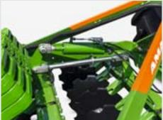
The hydraulic depth adjustment, which can be chosen as an option, offers huge comfort for the Catros and Catros Special. Changeable on the move, it allows the adjustment of the working depth from the tractor cab.
