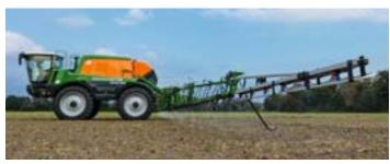
Plant protection systems: e.g. Pantera self-propelled sprayer
