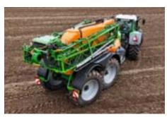
The combination of sprung drawbar, hydropneumatic suspension and axle steering come together to give an especially smooth, stress-free boom guidance and optimum driver comfort.
