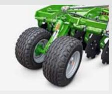
On Certos-2TX the working depth is adjusted steplessly and hydraulically via the support wheels from the tractor seat. The indicator scale for the depth is easily visible from the tractor seat and allows always the easy depth monitoring.
