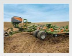
As special optional equipment for Cenius-2TX, the GreenDrill seeder box is available. This allows the combined soil tillage and sowing of catch crops in just one operational pass.
