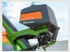
The ED can be equipped with one or two micro-granular applicators. In this way, during one pass, up to two micro-granules can be applied to the seed, depending on the machine type.
