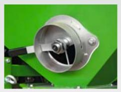
The emptying of the seed and fertiliser tanks is done quickly and easily via the optionally available quick emptying device which is attached to the tank and is easily accessible. By the use of some HT or drainage piping, the access can be extended to ease emptying.
