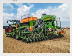
The GreenDrill 501, with 500 l hopper capacity, is suitable for sowing catch crops, fine seeds, undersown crops and spreading fertiliser in combination with the trailed AMAZONE soil tillage range or the Cirrus trailed drill combination.
