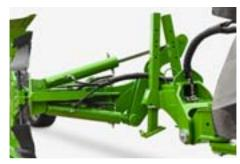
The new swing-arm system that forms the front connection between plough beam and turnover mechanism, ensures the maximum true track following and the optimum pull line of the combination. The turnover cylinders, with hydraulic end positioning damping, guarantee a smooth, sequenced turnover procedure for the plough.
