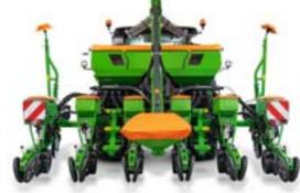
Precea 4500-2CC with a variable telescopic frame at a full working width
