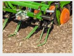
In order to cope with the ever-increasing sowing speeds, the RoTeC pro coulters feature an especially strong coulter bearing point. The Exact S following harrow provides good seed coverage, even under the most arduous of operating conditions and where copious amounts of straw prevail.
