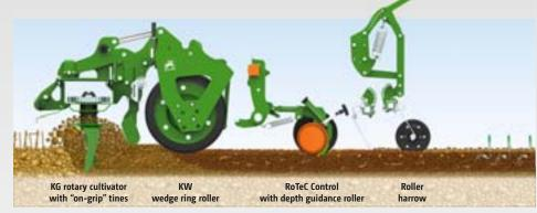
Because of the de-mixing effect coarser, soil particles remain on the surface. The fine soil remains in the sowing level creating superb germination conditions. In this way the seed is placed into the fine soil. The coarser parts on the surface protect from capping, drying out or erosion. The "Roller-Drill-System" with wedge ring roller, RoTeC Control coulter and roller harrow provides improved seed emergence and increased yields.
