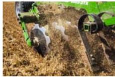
For levelling and better crumbling, a Crushboard in front or behind the disc rows is available as option. In this way, especially after ploughing, coarse clods on the surface can be broken up.
