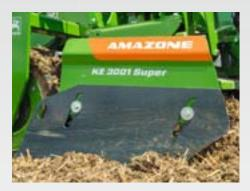
The side plates are mounted on a sprung suspension which allows them to yield upwards when stones are encountered. A long carrying arm and sturdy springs also make the KE Super reliable to use on stony, heavy soils. This applies also to all rotary cultivators.
