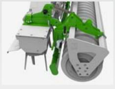
The levelling board levels the earth flow between the tines and the roller and presses obstacles downwards. Where larger obstacles prevail, the integrated overload safety enables the levelling board to give way in an upward direction.
