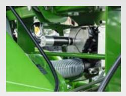
The seed metering is carried out via the electrically-driven metering unit underneath the seed hopper. When using different seeds, different metering cassettes are available which can then be quickly and easily exchanged.
