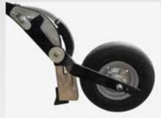
For a long service life the coulter tips are equipped with a hard metal coating. The comfortable depth setting means that adjusting the placement depth can be done in the shortest of times.
