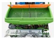
The hopper opening features a spacious 2.43 x 0.91 m so that the Centaya can be filled via big bags or via a front end loader without a problem. When filling via small sacks, the protective sieves in the seed hopper can be utilised as a loading aid.
