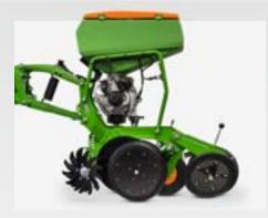
The PreTeC mulch seeding coulter has a maximum coulter pressure of 220 kg, using mechanical coulter pressure, and 400 kg using hydraulic coulter pressure. This ensures smooth running and even field emergence under the hardest of soil conditions.
