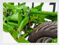
The setting of the plough tilt is done without tools and is adjustable individually for the right and left hand side.
