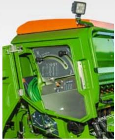
AMAZONE offers the SmartCenter, which provides a very simple and clear arrangement of the most important settings, in order to make operation even easier. The electric metering system can be quickly configured and calibrated centrally from the left-hand side.
