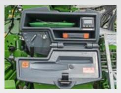
Via the SmartCenter, positioned to the left of the machine, the Centaya Super can be comfortably calibrated and adjusted from ground level. The digital weigh scales and a folding bucket are stored in the transport box to the side of the machine.
