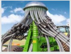
A useful system to assist the driver is the optionally available seed pipe monitoring which detects immediately any blockages down at the coulter and in the tube. Sitting directly behind the distributor head, sensors monitor the seed flow in the seed pipes.
