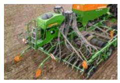
The pneumatic GreenDrill catch crop seeder box, when mounted on the trailed Cirrus sowing combination, allows the user to apply to the soil surface an additional medium during the sowing procedure. This could be in the form of either seed for under-sowing or for applying slug pellets.
