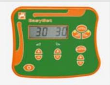
With the aid of the EasySet operator terminal, the left and right hand side outlet apertures can be set individually via a quick press of the soft key and so can be adjusted on the move.
