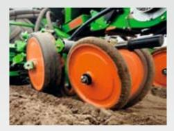
The two 500 mm diameter carrying rollers per sowing coulter run very smoothly thanks to their wide contact area and support the entire sowing unit. The pressure on the carrying rollers can be adjusted centrally and hydraulically and thus easily matched to the prevailing soil conditions.
