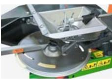
A high-quality charged-particle paint finish (car industry standard) is used on the hoppers and frame whereas the spreader unit, made completely of stainless steel, guarantees a long life and a high resale value.
