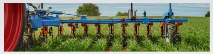
Low wear, e.g. by using HD versions of the soil-engaging metal, is becoming ever more important for hoe systems, due to increasing driving speeds and increasing work rate requirements. In order to decrease the length of time not working, or to simplify blade changing to suit different operating conditions, for example, a quick change knife system is becoming more and more considered as standard equipment. Maintenance-free bearings on the hoes also reduces machine downtime.
