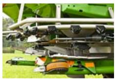
The ZA-TS spreaders can be equipped with the Argus system for spread fan recognition. Argus Twin, via radar sensors, permanently monitors both the left and right hand spread fans and then automatically corrects them, independently of one another, using the electrically-actuated delivery system if necessary.
