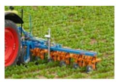
Precise camera and control technology leads to an enormous increase in output. Even row spacings as narrow as 12.5 cm can be detected by the camera. Thanks to the camera technology, driving speeds of up to 15 km/h are now possible without any problems.
