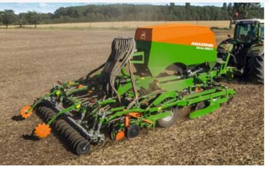
With the Minimum TillDisc corrugated disc segment, the Cirrus gets a new special option in place of the cultivation discs. On a row spacing of 16.6 cm, the ground, the harvest residues and also any green crop can be cut directly in front of the sowing coulters for a clean seed/soil contact.
