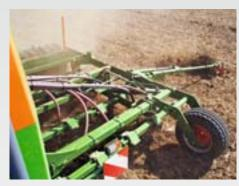
At 3600 I, the seed hopper on the Cayena is large, but still compact. This allows a clear view of the TineTeC coulters during use. The large hopper opening ensures the easy and rapid filling.
