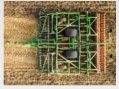
With the following tine segment, loosening of the deeper soil layers down to 30 cm is possible. However, shallow operation is also possible so that, under wet and arduous conditions, the tine tip runs just below the working depth of the disc harrow.
