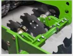
The disc harrow with its maintenance-free and uniquely angled discs ensures a superb quality and level seedbed. The working depth can be hydraulically adjusted during operation.
