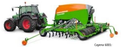
36 tine coulters, 16.6 cm row spacing – forward speeds of up to 15 km/h
