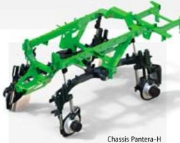
The special tandem chassis of the Pantera not only ensures the perfect adaptation to ground undulations, but also a high stability – of course, especially in sloping terrain. Thanks to the level-regulated, hydro-pneumatic suspension system the Pantera operator also enjoys the maximum level of comfort.
