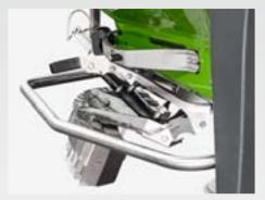
For the ZA-V with hydraulic shutter slide actuation the hydraulically actuated Limiter V border spreading system is available for side, border and water course spreading. Prior to spreading, the recommended working height of the Limiter V is fixed via a pin, depending on the border situation.
