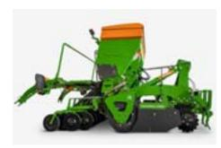
Thanks to the QuickLink quick coupling system, the CombiDisc can be removed with just a few hand clamps so that the mounted compact disc harrow can be readily used in solo operation for seedbed preparation.
