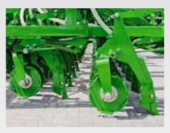
All the chisel openers are mounted on a parallelogram linkage. This prevents any reduction in the accuracy of the desired sowing depth even at different or changing forward speeds and in undulating ground conditions.
