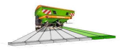
The 8 or 16 fold part-width section control of the ZA-V allows actuation of individual outer part-width sections.
