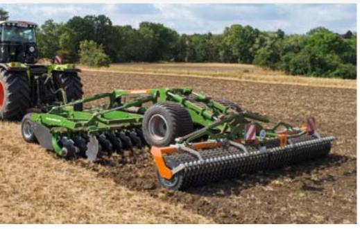
To ensure an even depth control of the machine, the Certos-2TX is guided at the rear via the following roller and up front via the support wheels.
