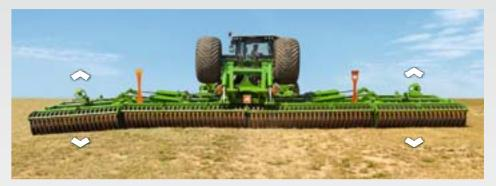
The Catros<sup>+</sup> 12003-2TS comes equipped with 510 mm diameter serrated discs making possible working depths from 5 down to 14 cm possible. The ContourFrame on the Catros<sup>+</sup> 12003-2TS is divided in four separate segments allowing each of them float. In this way the pressurised hydraulic system allows the individual soil contour following of each of the 4 segments.
