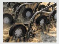
The ConTeC pro coulter excels itself, because of the trailing guide wheel, with its precise contour following. The coulter spacing, the 3 stagger layout of the coulters and the high frame height guarantees a blockage-free operation.
