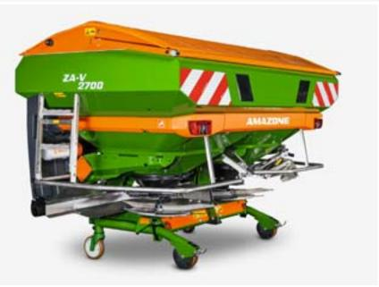
The strong frame and favourable centre of gravity position characterise the ZA-V as a robust mounted implement. The Super frame provides a payload of 3200 kg whereas the Ultra frame takes up to 4500 kg.
