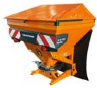
The E+S Hydro 751 winter salt spreader is equipped with a 750 litre hopper with stainless steel hopper tip, hydraulic spreading disc drive and a forward speed related spread rate regulation
