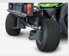
On the Profihopper SmartLine 4WDi, every wheel, due to accelerator pedal position and steering angle, is driven with the necessary speed for maximum traction. Especially in difficult operating conditions, the user benefits from the intelligent all-wheel drive.
