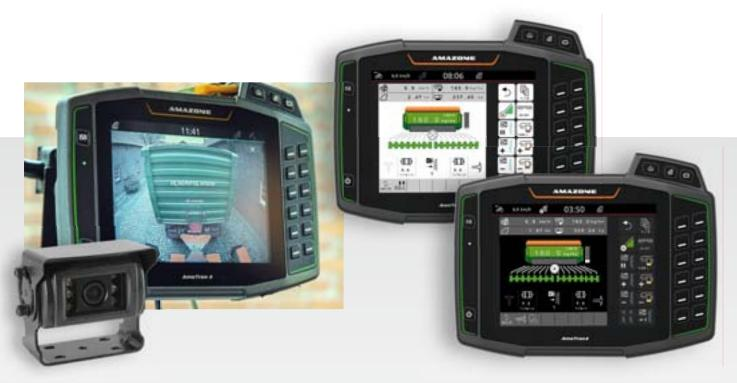
Automated AmaCam reverse driving recognition that gives direct access to a reversing camera and prevents dangerous situations
