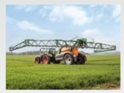
With Profi-fold or Flex-fold, all hydraulic functions, even independent, one-sided folding, are safely and simply carried out via the ISOBUS terminal from the tractor cab.
