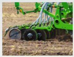
The TwinTeC<sup>+</sup> double disc coulter system features an infinitely variable hydraulic adjustment of the coulter pressure providing a wide setting range from 15 to 100 kg. In this way, the pressure can be matched quickly and simply to the changing soil conditions.
