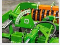
Adjustment of the working depth is carried out, very comfortably and as standard, via a hydraulic spool valve from the tractor cab ensuring that the working depth can be flexibly matched to the situation. This allows operation in the field to be as shallow as possible and, on the headlands and in deep wheel tracks, as deep as necessary.
