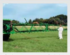
After the spraying operation is finished, with the aid of the spray lance on the wash down kit, any sprayer from AMAZONE can be thoroughly cleaned externally in the field.
