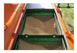
The Citan 12001-C and 15001-C offer the possibility to also place fertiliser together with the seed into the same furrow. Therefore the hopper is divided and can be filled either 2/3 with seed and 1/3 with fertiliser or maybe a second seed type. If the division in the hopper is not required, the hopper can be completely filled with just one seed type. The metering is carried out via Vario gearboxes which can meter seed rates from 1.5 to 400 kg/ha.
