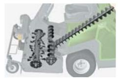
Due to the integrated PowerCompactor collection and conveying system, the cuttings are delivered immediately after mowing into a conveying auger system, compacted and collected in the collection hopper. This means that the Profihopper, in comparison with similar implements, offers higher conveying capacities and speeds, especially in tall grass.
