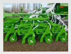
The 4-stagger arrangement of the opener units on the frame results in a large spacing between the openers to ensure excellent straw passage.
