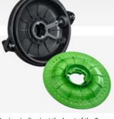
Precise singling is at the heart of the Precea. Metering is provided by overpressure. The seed and the entire metering unit are pressurised by a blower fan. Three strippers ensure that any excess seeds are removed, in order to prevent doubles. This results in very accurate singling, even at high driving speeds up to 15 km/h.
