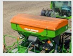
The roll-over hopper cover is easy to handle and protects the seed hopper from dust and rain.
