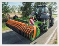
The new Catros<sup>XL</sup> is equipped with individually adjustable side discs. In the 3 and 4 m versions these discs can be simply folded in for road transport to maintain the relevant transport width.
