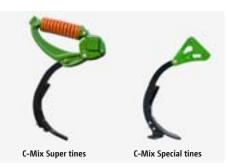
Together with the C-Mix Super pressure spring overload stone protection, the tine element in the centre of the machine provides a perfect working performance even when top soil deep loosening. In this way efficient and continuous operation is achieved even under the most arduous of conditions. The C-Mix Special tine with its shear bolt overload safety device is the alternative for light and medium-light soils without stones.
