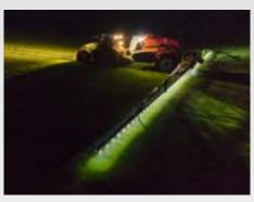
The optional LED individual nozzle lighting means that the illumination of the spray fan is targeted even more. Even the functionality of the last nozzle on the boom can be checked without a problem.
