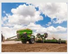
The trailed XTender-T is ideally suited to tractors without a three-point linkage or those with little lifting power. The running gear permits a support load from the attached implement of up to 4000 kg.
