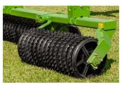
The AW rollers are available with either Cambridge or Crosskill rings in all working widths. The individual roller segments with their freely moving intermediate rings are mounted separately from each other in order to ensure outstanding self-cleaning and contour adaptation over the full working width.
