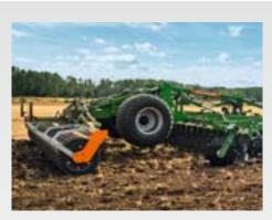
The integrated centre running gear results in the high manoeuvrability of Certos-2TX. To maintain a very smooth, comfortable ride and an optimum working performance, the Certos-2TX is fitted as standard with a drawbar shock absorbance system.
