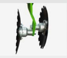
The 2-row disc harrow loosens, crumbles and levels the seedbed prior to the seed placement. The discs of the CombiDisc are aggressively angled, 14° at the front disc row and 12° at the rear disc row. This angle ensures the optimum levelling of the seedbed.
