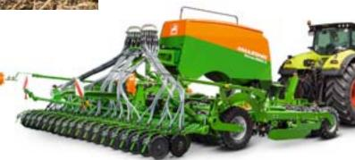
Cirrus 6003-2 sowing combination with TwinTeC<sup>+</sup> double disc coulters
